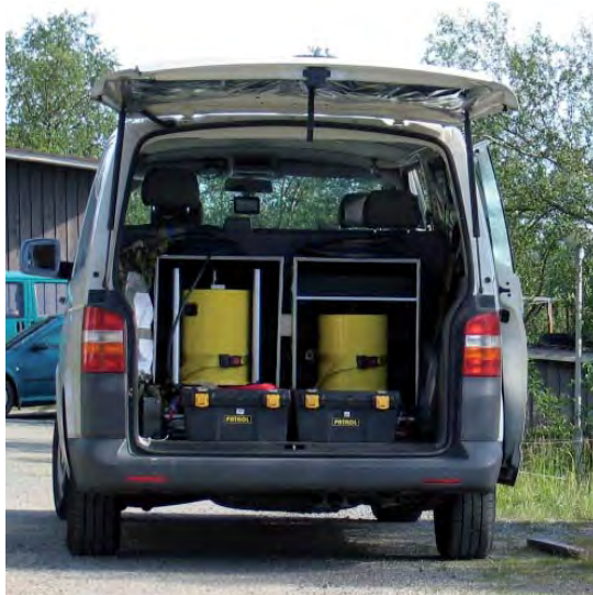
Fig. 4. The A10-020 in the mobile gravity laboratory; left – dropper and interferometer unit in transport position, right – the electronics unit
