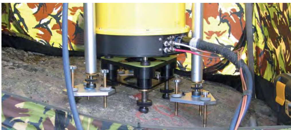
Fig. 6. Setup under rough field conditions, with the IGiK-constructed special stands for the dropper legs
