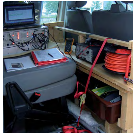
Fig. 4. The A10-020 in the mobile gravity laboratory; left – dropper and interferometer unit in transport position, right – the electronics unit
